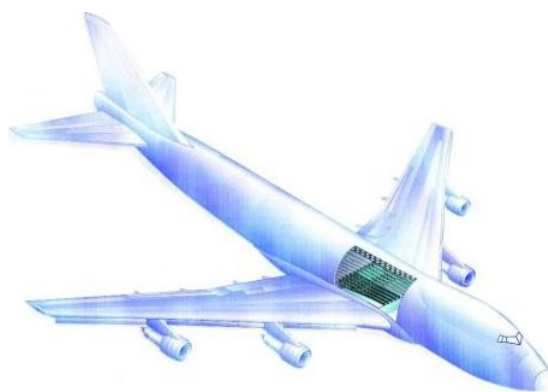
Figure 1: A 747, cutaway to show the top of the center wing fuel tank, just beneath the passenger cabin. 1
